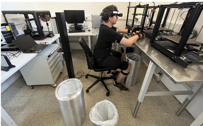
Fig. 4: Simulating Signal Distortions with Metallic Objects
